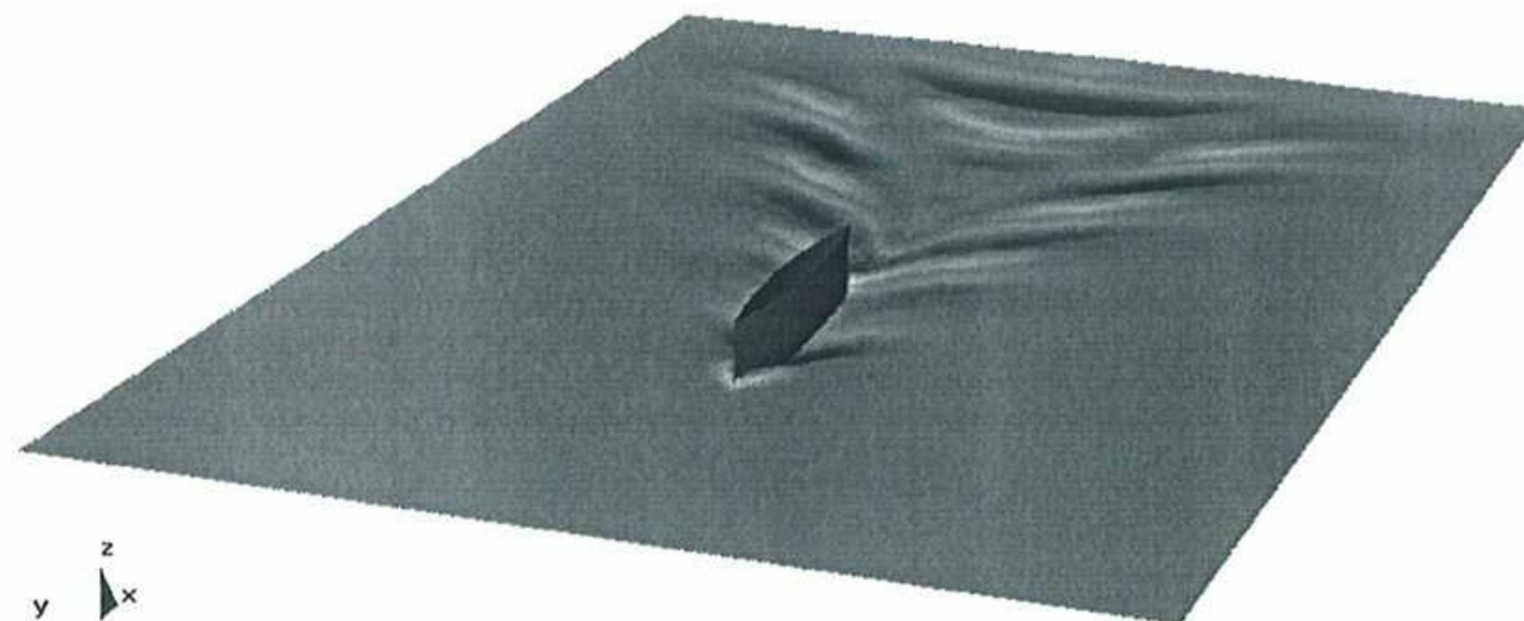
Figure 7: Wigley hull. a) Pressure distribution and mesh deformation of the wigley hull (free model). b) Numerical and experimental body wave profiles. c) Free surface contours for the truly free ship motion.
