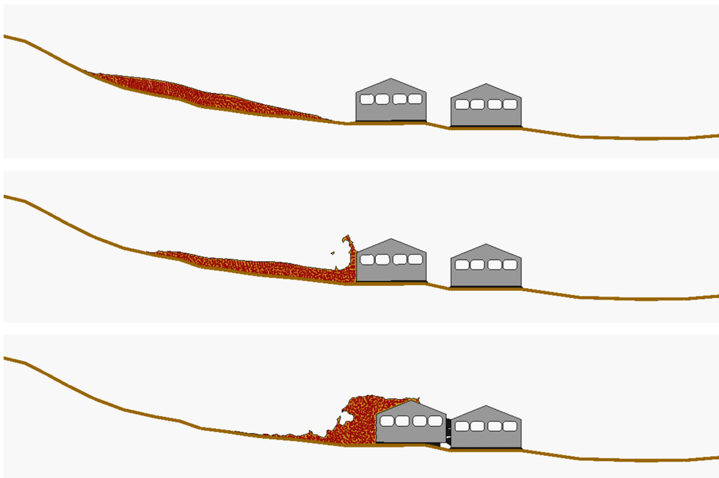
Fig. 11 Landslide falling on two constructions 2D simulation using PFEM
