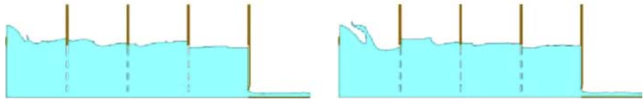
Figure 30. Sluice gate. Model 2. Simulation of the flow at different instances
