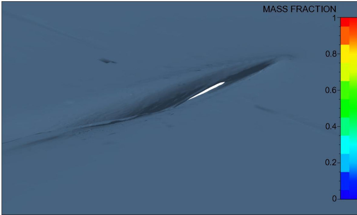
Fig. 30 Oar blade and the free surface around it.
