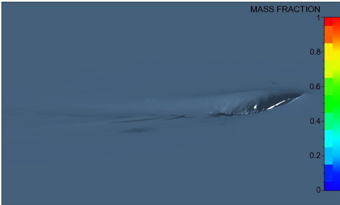
Fig. 31 Oar blade and the free surface around it when the blade starts turning.
