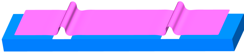
Figure 1.7: Position of fold controlled by patterning the substrate. The adhesion energy is removed in the strip beneath the fold so that the fold can be directed here
