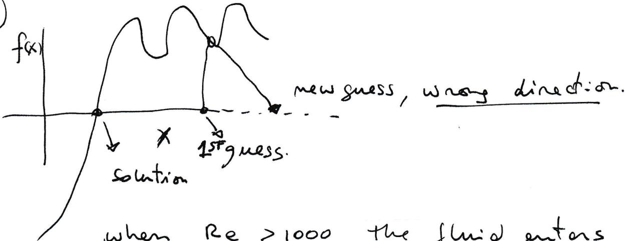
when  $Re > 1000$  the fluid enters transition regime and becomes chaotic. It is reasonable that gradient methods should fail to find a solution. A combined approach (Picard first and Newton second) might be the best approach.
