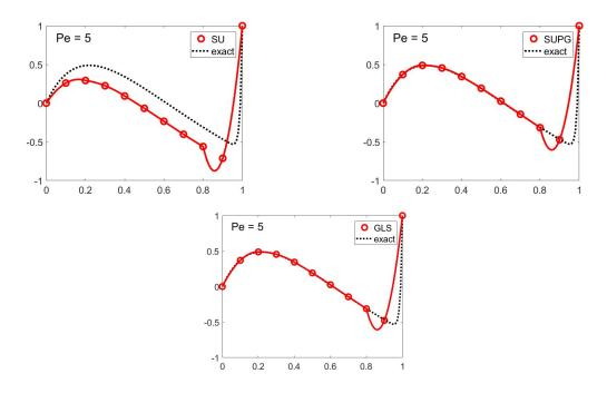
Clearly, having a source term made things different as it affects the formulation. The SU fails to obtain exact nodal values. However, the SUPG and GLS methods have almost exact nodal values and have similar solution even though they have different stabilization terms.
