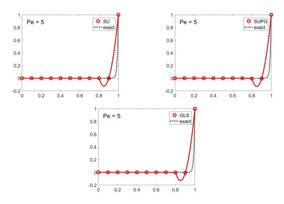
Clearly, the solution of all the methods is identical. Although, the formulation of the 3 methods is different, having no source term and the behaviour of the problem led to similar solution. Almost exact nodal values are obtained by all of the methods.
