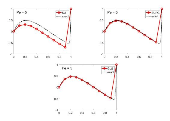
It should be noted from the results that GLS and SUPG are identical since the  $2^{nd}$  order derivative is zero due to using linear shape functions. Moreover, GLS and SUPG provide exact nodal solution. On the contrary, SU doesn't result in exact nodal values; its result was different due to the existence of a source term. SU doesn't take into account the residual in the formulation; that's why it's not a consistent method.
