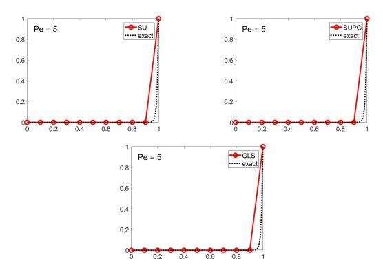
It should be noted that the three methods lead to the same exact result. The 3 methods are identical since the term that has  $2^{nd}$  order derivative becomes zero due to using linear shape functions and the source term is zero which will lead to the same equation for all of them. These method with linear elements lead to exact nodal values as shown.
