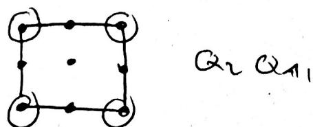
The problem is that with this configuration the pressure and velocity are interpolated at different nodes, and some people prefer to use Q<sub>1</sub> Q<sub>1</sub> elements and stabilization techniques.
