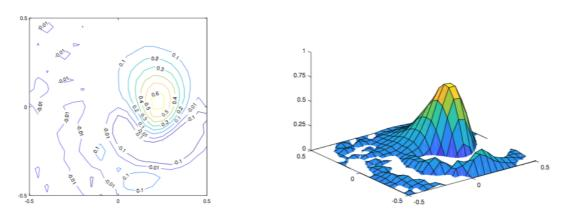
In this figure we can see the implementation of CN + Galerkin with Lumped Mass matrix
