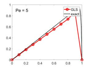
We can see that the Galerkin method starts oscillating in the very beginning and when we implement the Upwind we see that it stabilizes a lot the solution. For SUPG and GLS in linear elements we get the same exact result. The piece of code we added to approximate the solution is just adding the source term to the equation such as:
