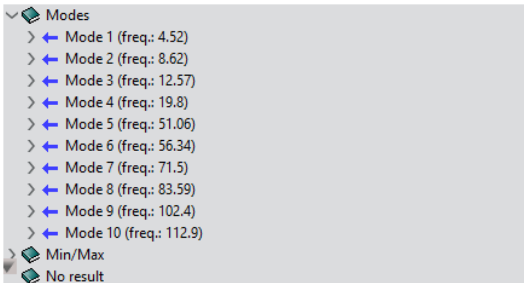
Figure 28: Result: first ten modes of vibration with natural frequencies
