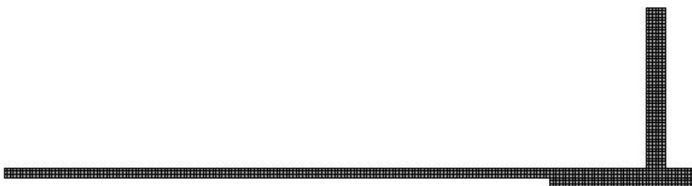
Figure 5: Structured mesh generation with linear quadrilateral mesh elements
