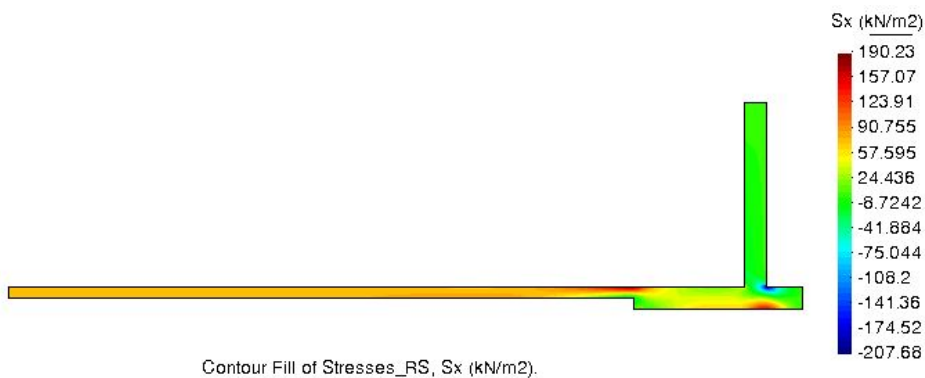
Figure 8: Results: Plot of stresses S_x
