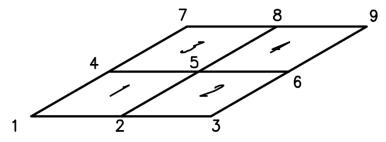
The length of the sides of the rectangular shape are 1. The boundary condition in the four edges are SS. So, imposing a quadratic displacement field (can be represented with the MCZ)
