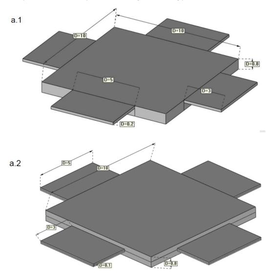
b) Define and verify a patch test mesh for the MCZ element.
