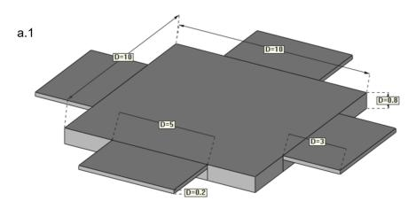
The first structure shows the problem of offset between the elements (the plates don't share the same middle plane). Two solutions can be used to model this structure.
