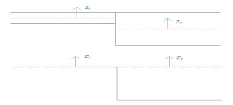
The second possibility is to use a rigid element that connects the two offset middle planes. In this case, the modeling process is more complex but has a more specific physical meaning.
