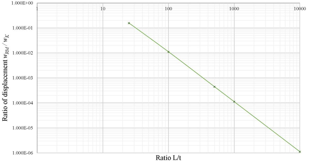
Fig. 2 – Comparison of maximum deflection predicted by MZC and Reissner-Mindlin plate elements
