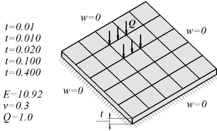
Fig. 1 – Boundary conditions and material properties
