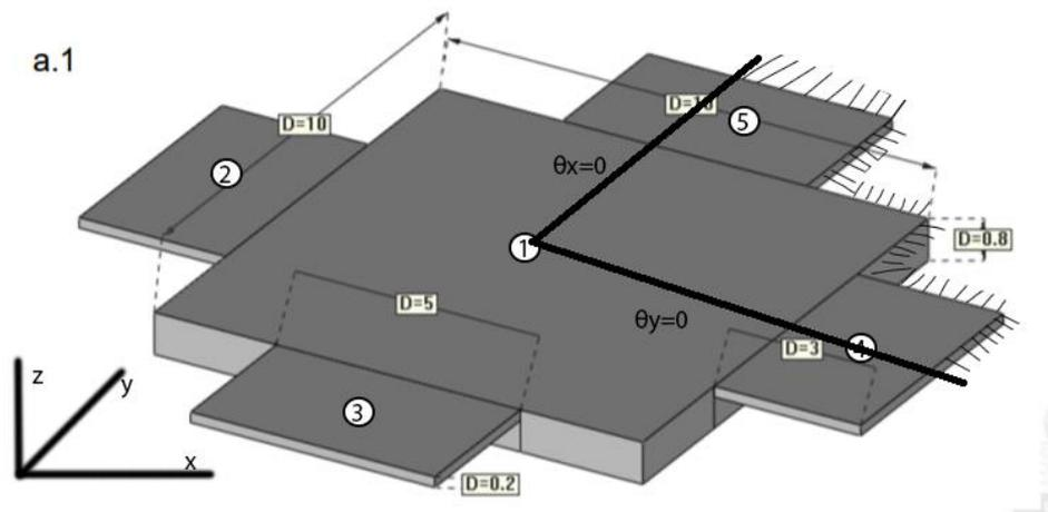
b) Define and verify a patch test mesh for the MCZ element.
