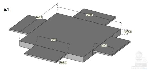
To begin with, we determine that this structure will be considered as a 5 different elements. To do this, it will be necessary to divide every side of the main square in 4, so we can make coincide the rectangular elements to it.
