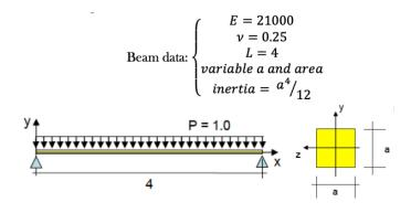
We will analyze the problem for each case mentioned (vary by a) and the results will be compared by means of a graph representing the displacement values (y direction), the maximum moment and cut for each type of element with respect to a / L.
