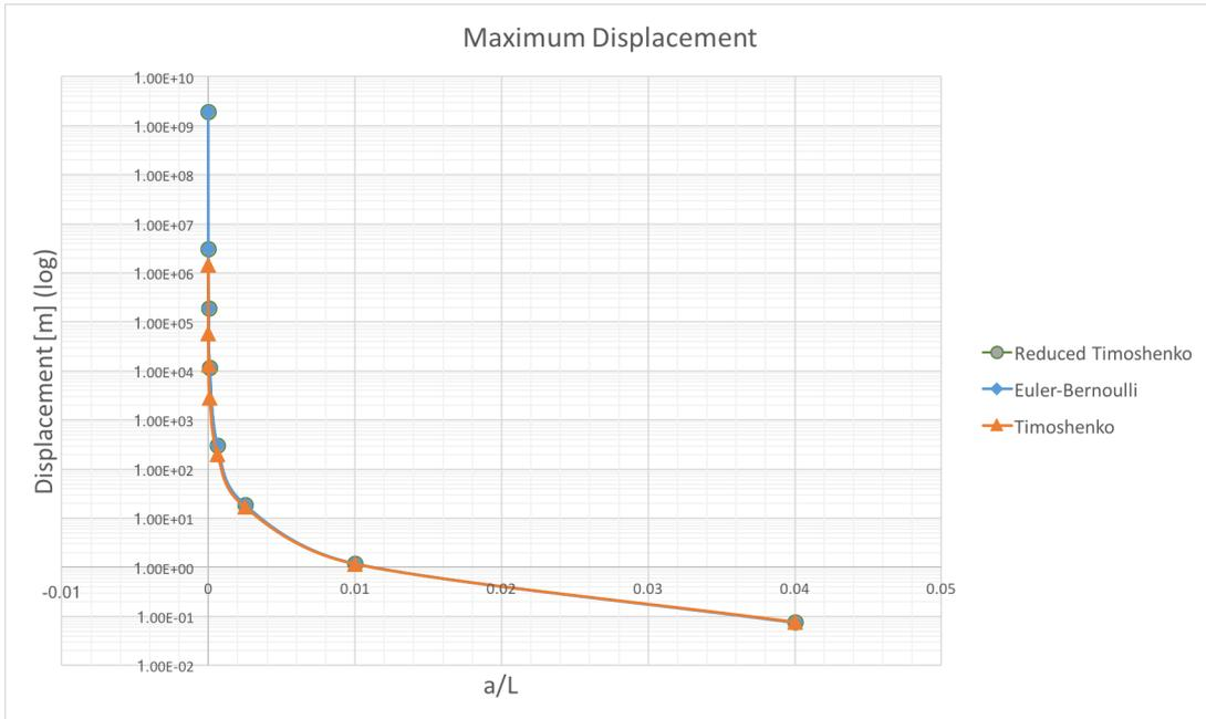
Figure 0.2: Displacement comparison between the EB, Timoshenko and Reduced Timoshenko.
