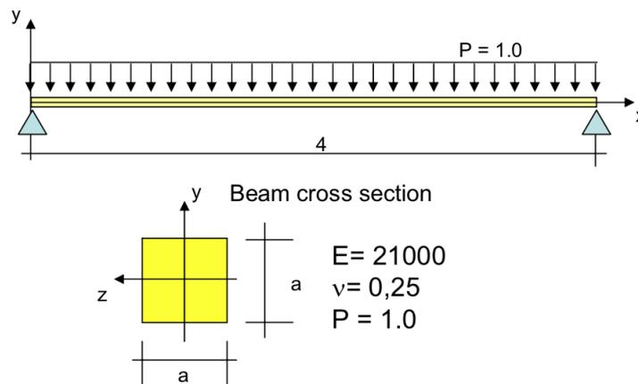
Figure 0.1: Geometry of the beam, load and mechanical properties.
