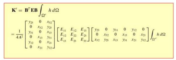
and write a simple script in Matlab to compute the stiffness matrix for the linear Turner triangle. The script is attached at the next page and the resulting stiffness matrix is
