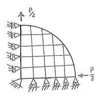
(c) In this case it can be define the anti-symmetry line, which is a horizontal line that divide the structure in two parts. We are using only half of the structure. According to the BC we impose no displacement in the direction of the line for the nodes contained in the anti-symmetry line.
