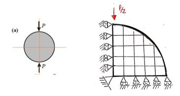
(b) In this case we can work only whit a quarter of the total structure but it is possible to define symmetry lines and also anti-symmetry lines, which have 45° grades. According to BC, for the symmetry case we have the same conditions as the previous case; for the anti-symmetry case the nodes corresponding with the centrer of the cylinder has no displacement, and the nodes on the anti-symmetry lines have no displacement in the lines directions.
