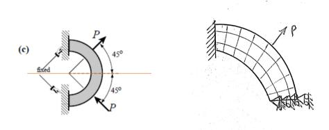
(d) In this case we can define two symmetry lines, like the first case (a). According to the BC those nodes in the symmetry lines, will have displacement in the corresponding line direction.
