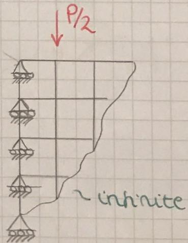
For element c) the part is restrained against movement in the x-direction because of the forces in x-direction nullify each other for the two halves.
