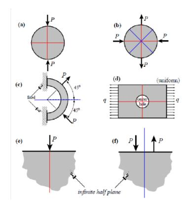
2. Having identified those symmetry/antisymmetry lines, state whether it is possible to cut the complete structure to one half or one quarter before lying out a finite element mesh. Then draw a coarse FE mesh indicating, with roller or fixed supports, which kind of displacement BCs you would specify on the symmetry or antisymmetry lines.
