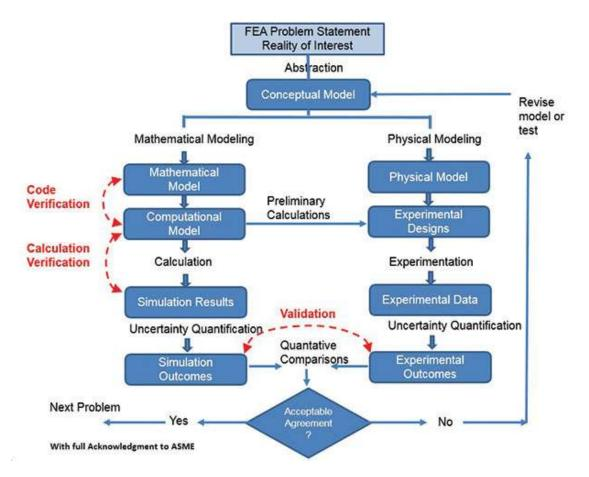
The early planning and assessment of the applicability of both the FEA model simulation methods and the test program to the real world structure and environment is done formally. It is also an integrated process between analysis and test disciplines.
