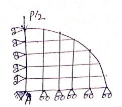
As the structure is doubly symmetric in both geometry and Loading, gt is exident that no y displacements are possible borc points on the X aruis and no X displacements are possible borc any points on the y arus.
