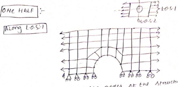
The y displacements of the nodes of the structure on the X and and zero. To prevent rigid body notion in the X direction, both the Xir displacements of the node A are constrained.
