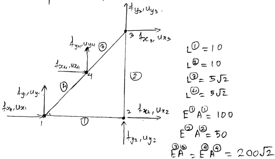
Here, we are calculating the element stiffness matrix for each element, using the standard formula
