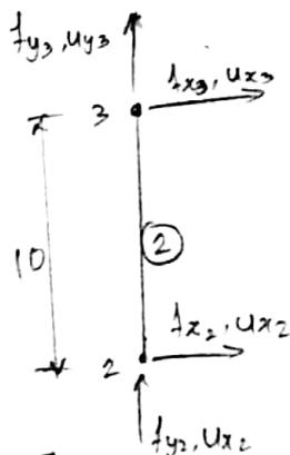
$$\begin{bmatrix} f_{x2}^{\textcircled{2}} \\ f_{y2}^{\textcircled{2}} \\ f_{x3}^{\textcircled{2}} \\ f_{y3}^{\textcircled{2}} \end{bmatrix} = 5^4 \begin{bmatrix} 0 & 0 & 0 & 0 \\ 0 & 1 & 0 & -1 \\ 0 & 0 & 0 & 0 \\ 0 & -1 & 0 & 1 \end{bmatrix} \begin{bmatrix} u_{x2}^{\textcircled{2}} \\ u_{y2}^{\textcircled{2}} \\ u_{x3}^{\textcircled{2}} \\ u_{y3}^{\textcircled{2}} \end{bmatrix} \quad \left( \frac{EA}{L} \right)^{\textcircled{2}} = \frac{50}{10} = 5$$
