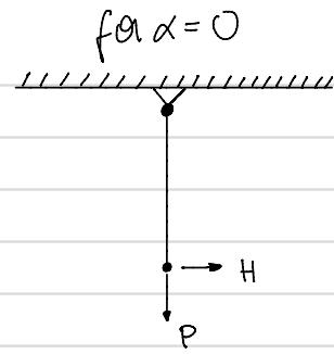
The solution for the axial forces "blow up" due to the infinite displacement in x direction.
