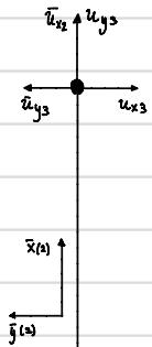
$$\begin{bmatrix} \bar{f}_{x_1} \\ \bar{f}_{y_1} \\ \bar{f}_{x_3} \\ \bar{f}_{y_3} \end{bmatrix} = \frac{EA}{L} \begin{bmatrix} 1 & 0 & -1 & 0 \\ 0 & 0 & 0 & 0 \\ -1 & 0 & 1 & 0 \\ 0 & 0 & 0 & 0 \end{bmatrix} \begin{bmatrix} \bar{u}_{x_1} \\ \bar{u}_{y_1} \\ \bar{u}_{x_3} \\ \bar{u}_{y_3} \end{bmatrix}$$
