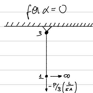
The horizontal displacement "blow up" due to the lack of equilibrium of momentum around node 3.
