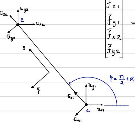
$$\begin{bmatrix} \bar{f}_{x_1} \\ \bar{f}_{y_1} \\ \bar{f}_{x_2} \\ \bar{f}_{y_2} \end{bmatrix} = \frac{EA}{L/c} \begin{bmatrix} 1 & 0 & -1 & 0 \\ 0 & 0 & 0 & 0 \\ -1 & 0 & 1 & 0 \\ 0 & 0 & 0 & 0 \end{bmatrix} \begin{bmatrix} \bar{u}_{x_1} \\ \bar{u}_{y_1} \\ \bar{u}_{x_2} \\ \bar{u}_{y_2} \end{bmatrix}$$
