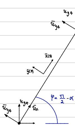
$$\begin{bmatrix} \bar{f}_{x_1} \\ \bar{f}_{y_1} \\ \bar{f}_{x_4} \\ \bar{f}_{y_4} \end{bmatrix} = \frac{EA}{L/c} \begin{bmatrix} 1 & 0 & -1 & 0 \\ 0 & 0 & 0 & 0 \\ -1 & 0 & 1 & 0 \\ 0 & 0 & 0 & 0 \end{bmatrix} \begin{bmatrix} \bar{u}_{x_1} \\ \bar{u}_{y_1} \\ \bar{u}_{x_4} \\ \bar{u}_{y_4} \end{bmatrix}$$
