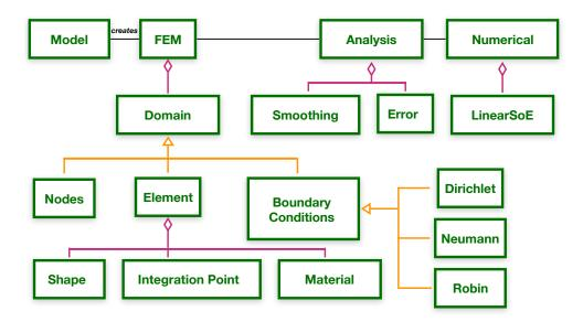
Figure 2: Hierarchy diagram showing inheritance and aggregation with additional classes
