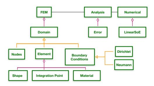
Figure 1: Hierarchy diagram showing inheritance and aggregation.
