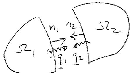
$$\underline{t}_1 + \underline{t}_2 = 0 \quad \text{Weakly} \quad \underline{n}_1 \cdot \underline{q}_1 + \underline{n}_2 \cdot \underline{q}_2 = 0 \quad \text{Weakly}$$
