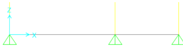
Figure 16: Hinged boundary condition
