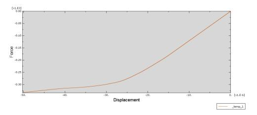
PLASTIC MATERIAL: f<sub>y</sub> (ε<sub>y</sub> = 0) = 460 MPa; f<sub>y</sub> (ε<sub>y</sub> = 0.002) = 520 MPa. The slope is steeper in the plastic part than in the previous case and the forces are higher for the same displacement as it can be shown in the forcedisplacement graphics.
