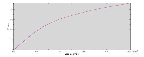
At the beginning, they work in the elastic range and they curve is quite similar. When the material exceeds the elastic limit the force gradient decreases. For elastic material continues growing in the same way withstanding a horizontal force of 490 N. However, the plastic material reaches lower values at the end of the step (<250 MPa).
