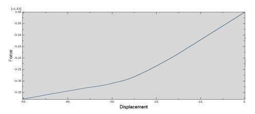
In conclusion, the first part is similar in all three cases because they are in the elastic range ( $f_y = 460$  MPa), therefore the force increase linearly. The plastic part is different especially between the first and the other cases. The force doesn't increase in the
