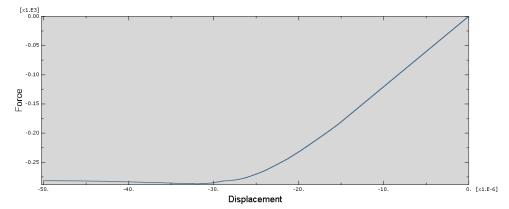
PLASTIC MATERIAL: f<sub>y</sub> (ε<sub>y</sub> = 0) = 460 MPa; f<sub>y</sub> (ε<sub>y</sub> = 0.005) = 520 MPa.
