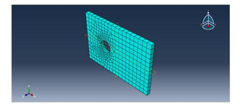
The response of the point under elastic condition should be linear and, as it was expected, the force rise gradually as a result of increasing the displacement. This means that the plate work in the elastic range. The force will grow infinitely while continuing increasing the displacement, because only elastic parameters are defined in the model.
