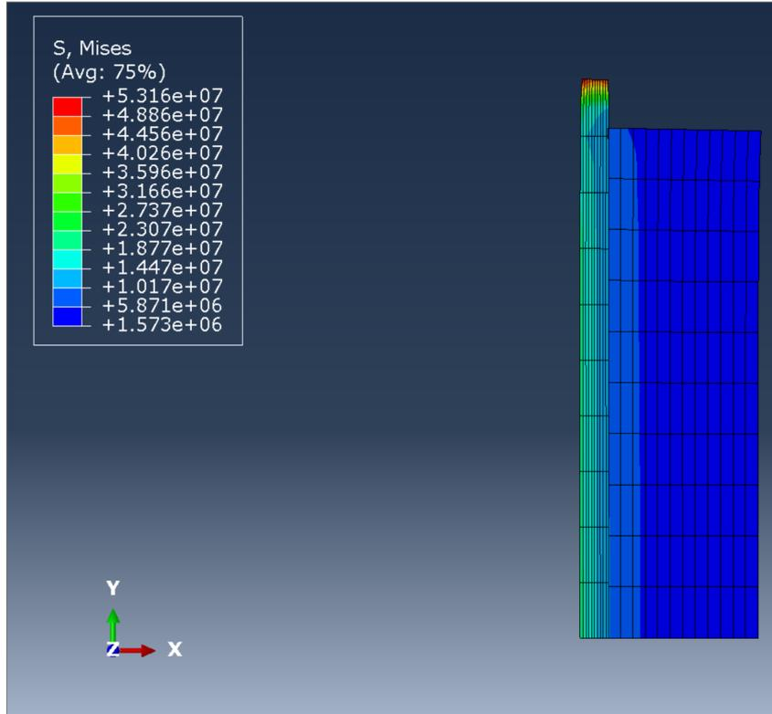
Figure 9: Von Mises stress distribution over a temperature-dependent concrete Young's Modulus.
