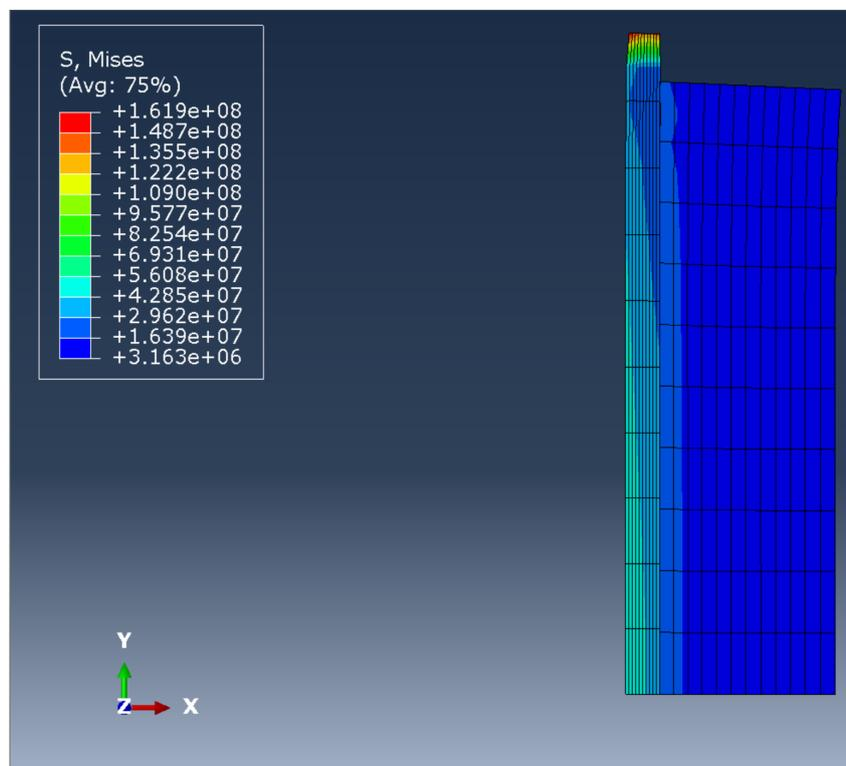
Figure 8: Von Misses stress distribution over the pile for an inner steel surface temperature of 90°C.
