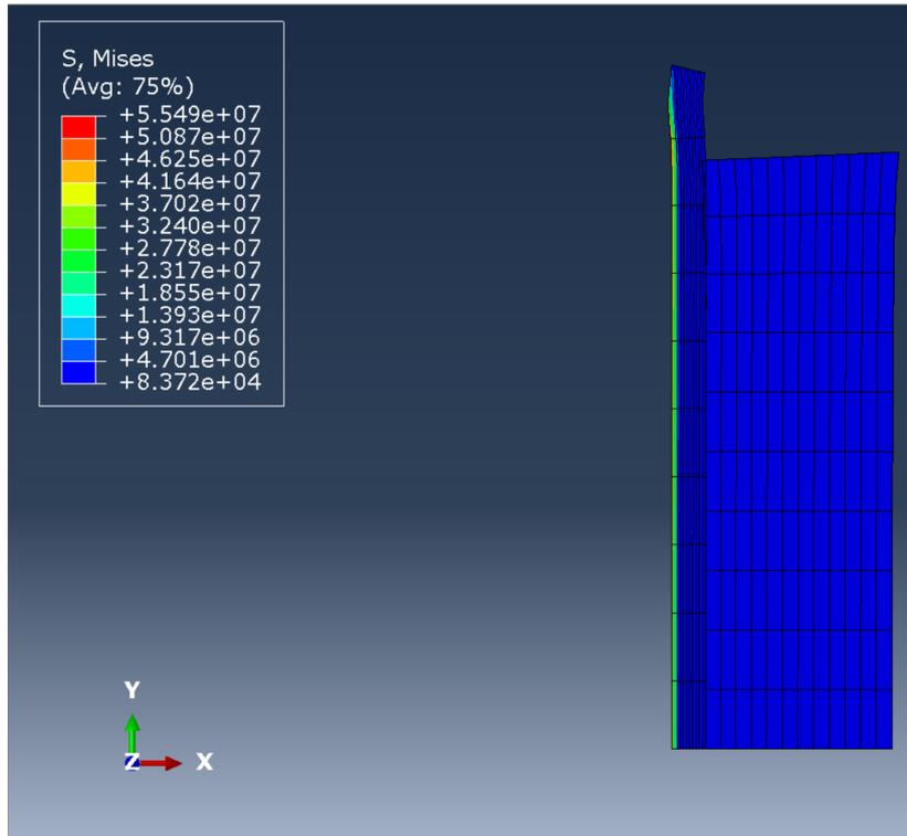
Figure 6: Von Mises stress distribution over the pile. Mechanical and thermal loads considered. Temperature in the inner surface of the pile.
