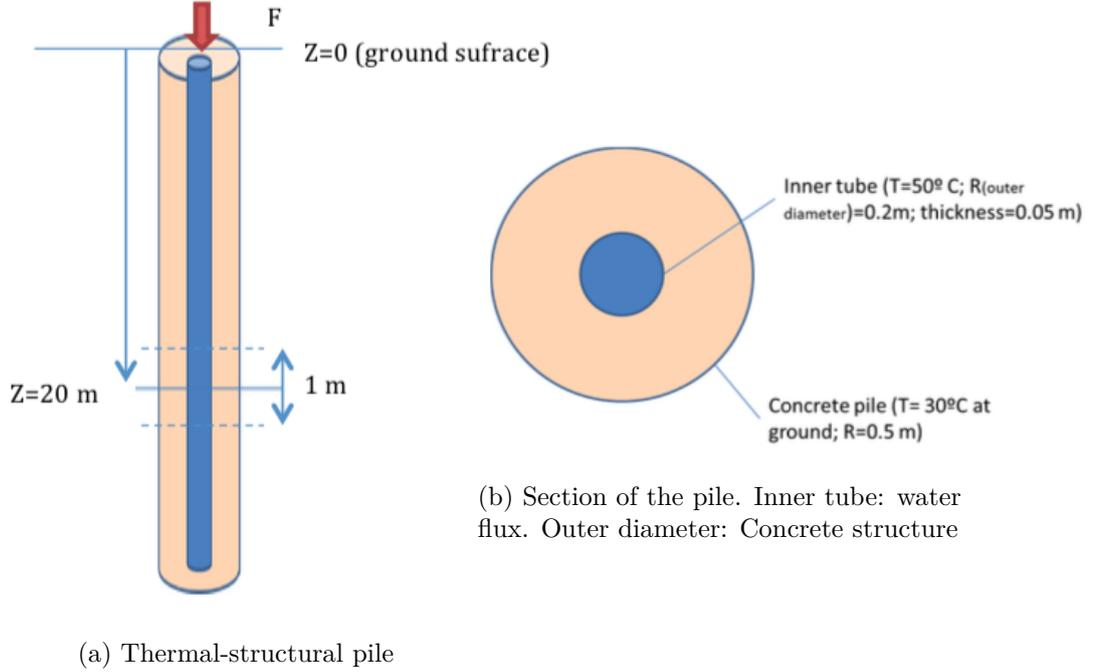
Figure 2: Pile geometry.
