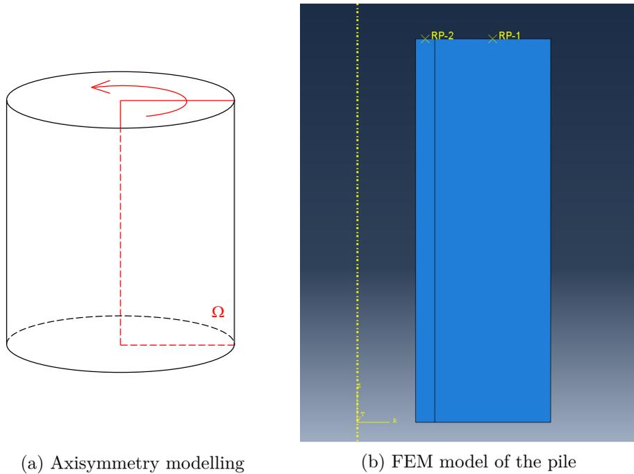
Figure 3: Pile model.
