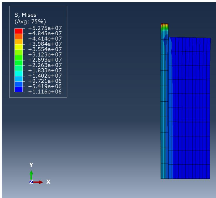
Figure 7: Von Mises stress distribution over the pile. Mechanical and thermal loads considered. Temperature applied to the whole steel width.
