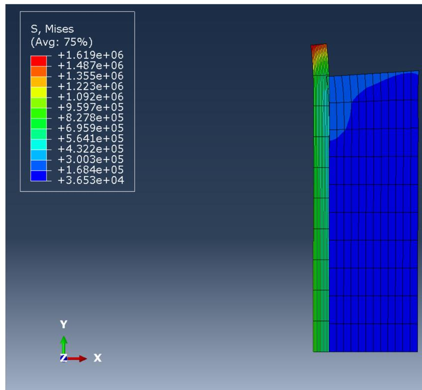
Figure 5: Von Misses stress distribution over the pile. Mechanical loads considered.
