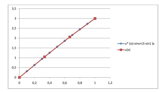
As we can see from the table and the graph, the approximate solution is equal to the exact solution. Two displacements  $u_2$  and  $u_3$  obtain the difference between the exact solution and the FEM is 0 and 0.0001 respectively. The approximations converge with a minimum error of 0.01% in the case of  $u_3$  and 0% in  $u_2$ . The exact solution can be approximated by a linear function (FE 2 node mesh with three elements).
