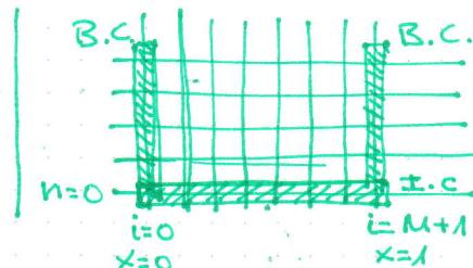
$$\left. \begin{aligned} \frac{\partial u}{\partial t} \Big|_{i,i}^{n+1} &= \frac{u_i^{n+1} - u_i^n}{\Delta t} \\ \frac{\partial u}{\partial x} \Big|_{i,i}^{n+1} &= \frac{u_{i+1}^{n+1} - u_{i-1}^{n+1}}{2\Delta x} \end{aligned} \right\} \rightarrow \frac{\partial u}{\partial t} = -a \frac{\partial u}{\partial x} ; \quad \therefore \frac{u_i^{n+1} - u_i^n}{\Delta t} = -a \frac{u_{i+1}^{n+1} - u_{i-1}^{n+1}}{2\Delta x}$$
