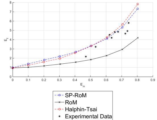
Figure 4: Relative transversal stiffness  $E_f/E_m$  vs. fibre volume fraction  $V_f$ . Comparison between the results given by the proposed method, experimental data, ROM and HalpinTsai equation.
