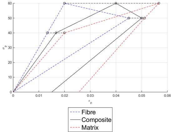
Figure 3: Serial stress (MPa) vs. serial strain curves for the composite and component materials under parallel deformation-controlled loadunload testing.
