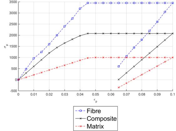
Figure 2: Parallel stress (MPa) vs. parallel strain curves for the composite and component materials under parallel deformation-controlled loadunload testing.
