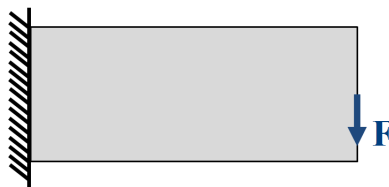
Figure 4.7: Schematic drawing of a cantilever beam with homogeneous material distribution
