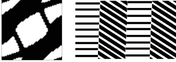
Figure 5.32: On the left, an optimal topology of a square RVE, on the right, a rank-2 laminate micro-structure. The Computational Vademecum can be improved by considering all kind of micro-structures (not only square RVEs). In the case of compliance, it can be seen that the optimal values are achieved when considering rank-2 laminates. [7].
