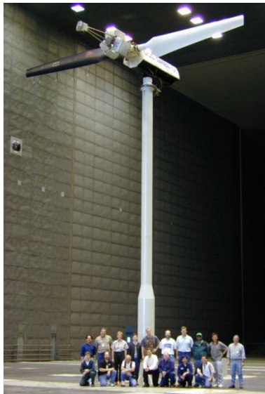
NREL-Phase VI-Experiment: 10 m diameter test turbine in NASA Ames wind tunnel
