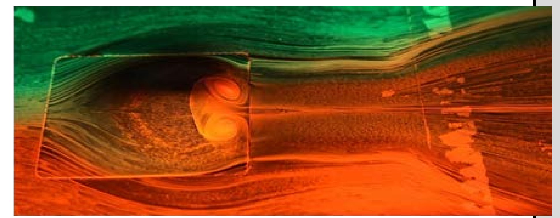
3D bumps for boundary layer control
